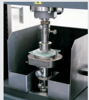
Fig. 14: Double ring flexure test
