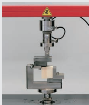
Fig. 13: Shear test on wood
