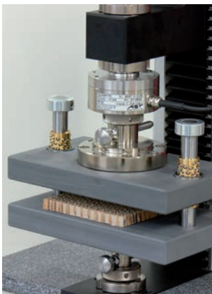
Fig. 5: Compression test on cardboard
