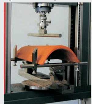
Fig. 16: Test on roof tiles
