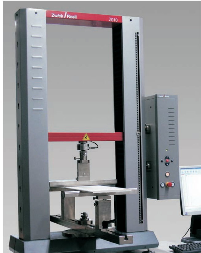
ProLine Z010 with 3-Point flexure test on plasterboard
