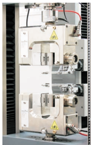
Fig. 3: Pneumatic grips 5 kN
