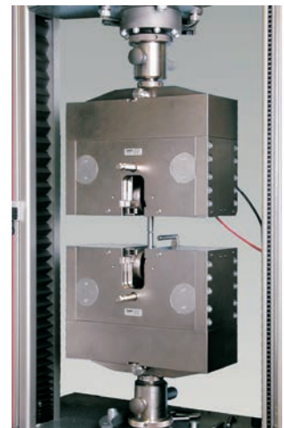
Fig. 4: Pneumatic grips 50 kN
