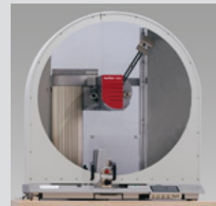
Fig. 4: HIT50P electrically interlocked safety device
