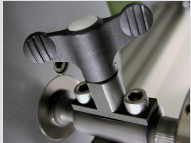
Fig. 1: The pendulum is easily changed by means of a quick release mechanism, eliminating the need for tools.
