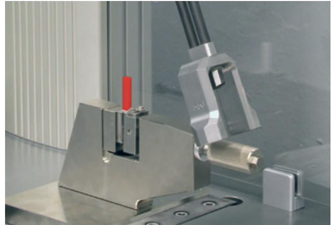
Fig. 1: Test with the manual Izod fixture clamp
