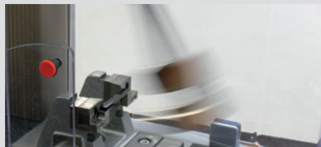
Fig. 3: HIT25P performing a Charpy impact test
