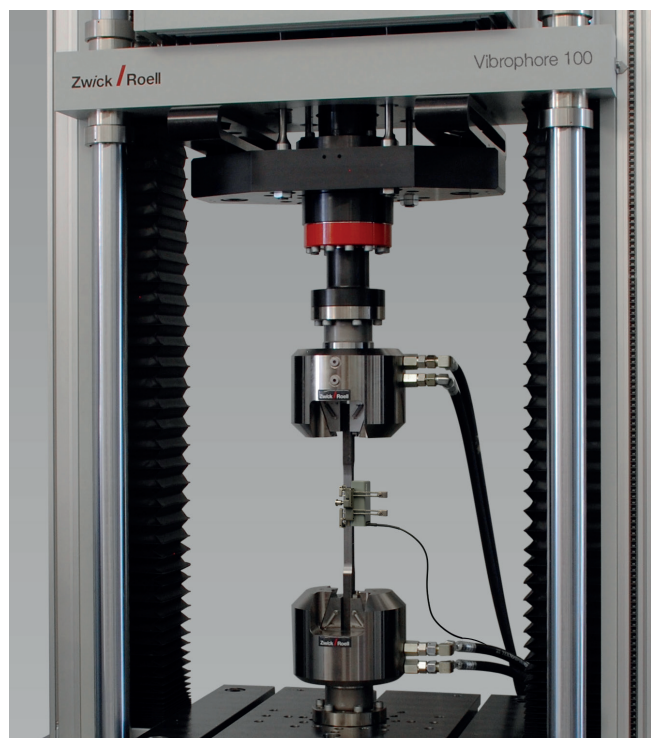
Fig. 2: Integration of makroXtens extensometer (top) and Clip-on extensometer (bottom) for static tensile tests
