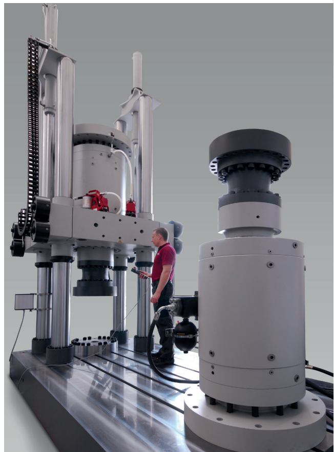
Fig. 3: Servohydraulic test portal for testing aircraft components
