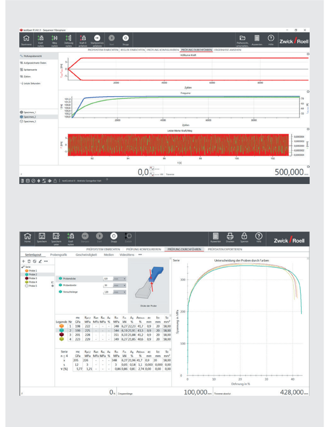
Fig. 2: The Vibrophore can be used for dynamic (top) and static (bottom) tests
