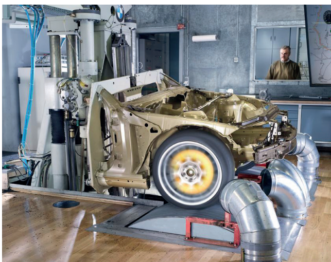
Fig. 1: Multi-axis test rig for follow-up tests (Image: © IABG)
