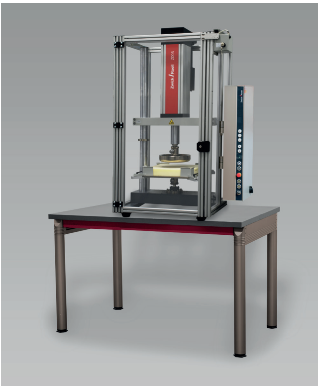
Fig. 1: Electromechanical servo testing actuator for fatigue tests on foam materials
