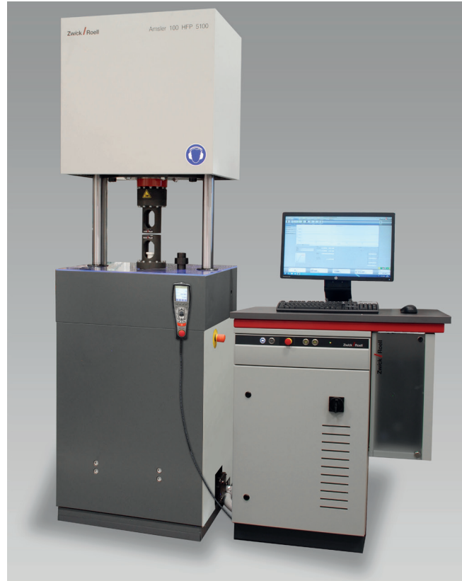
Fig. 2: Modernization of a Vibrophore with testControl II
