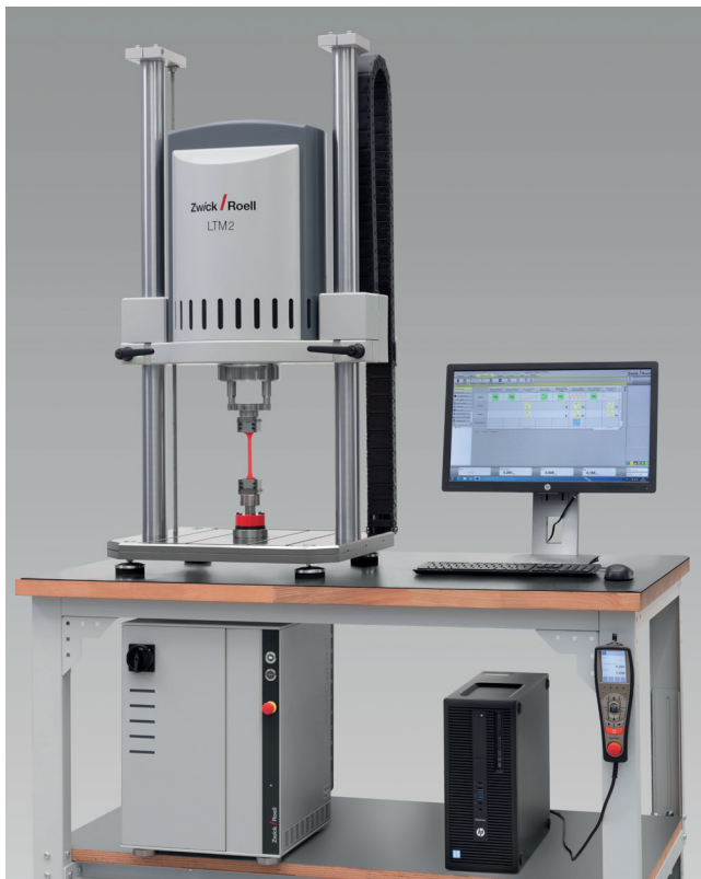
Fig. 1: LTM 2 testing system as table-top model
