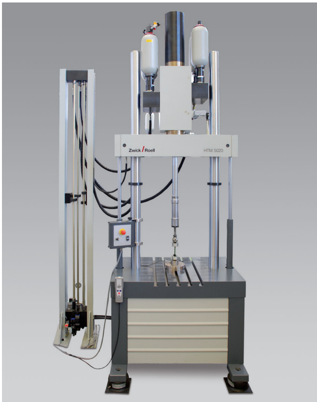
Fig. 1: HTM 5020 high-speed testing machine
