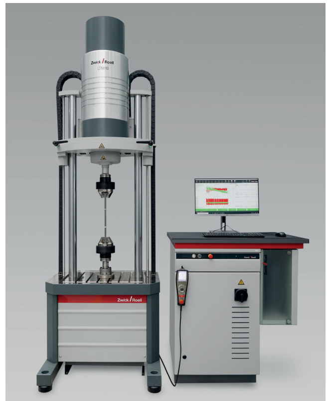
Fig. 3: LTM 10 linear testing system with torsion drive
