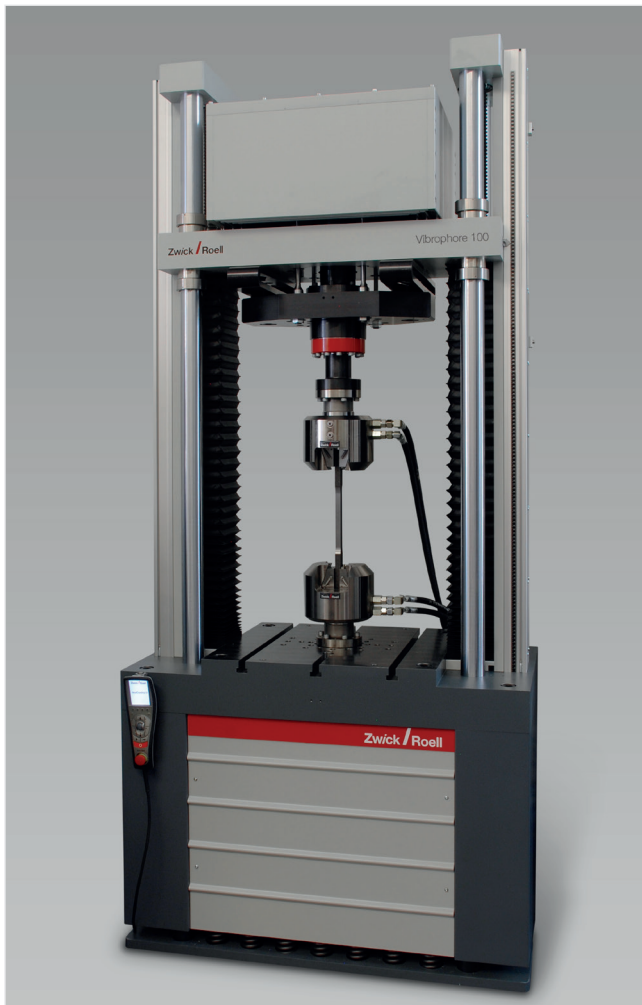
Fig. 1: Vibrophore 100 high-frequency pulsator with hydraulic wedge grips
