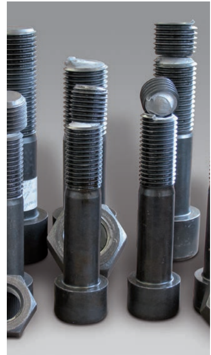
Fig.3: Bolts after testing
