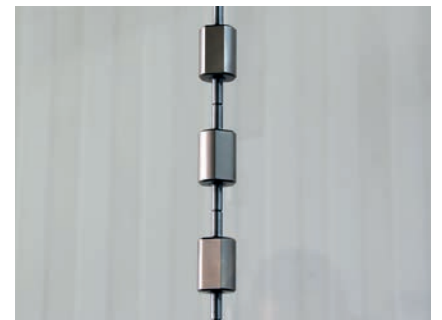
Fig.3: Testing for hydrogen embrittlement as per ASTM F519
