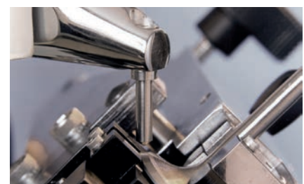
Fig.3: Rockwell test on hot-extruded engine valves
