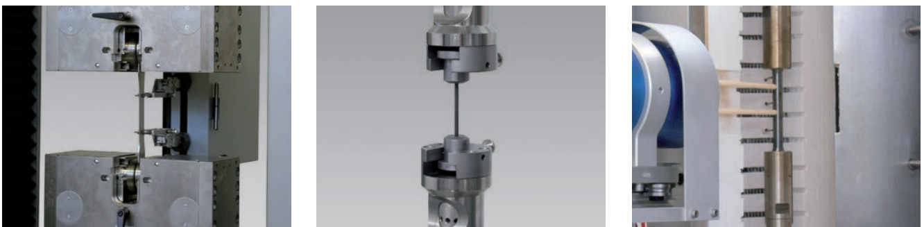
Fig.3: Pneumatic grips, dumbbell/screw/threaded-end grips, high-temperature grips
