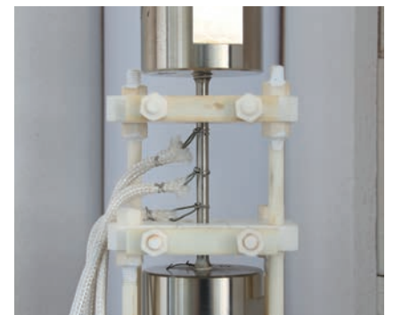
Fig.4: Gaged specimen for creep tensile test (extensometer and thermocouples)
