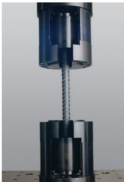
Fig.2: Specimen grips and specimen grouting for rebars
