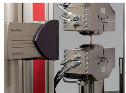
Fig. 6: laserXtens Compact for short specimens
