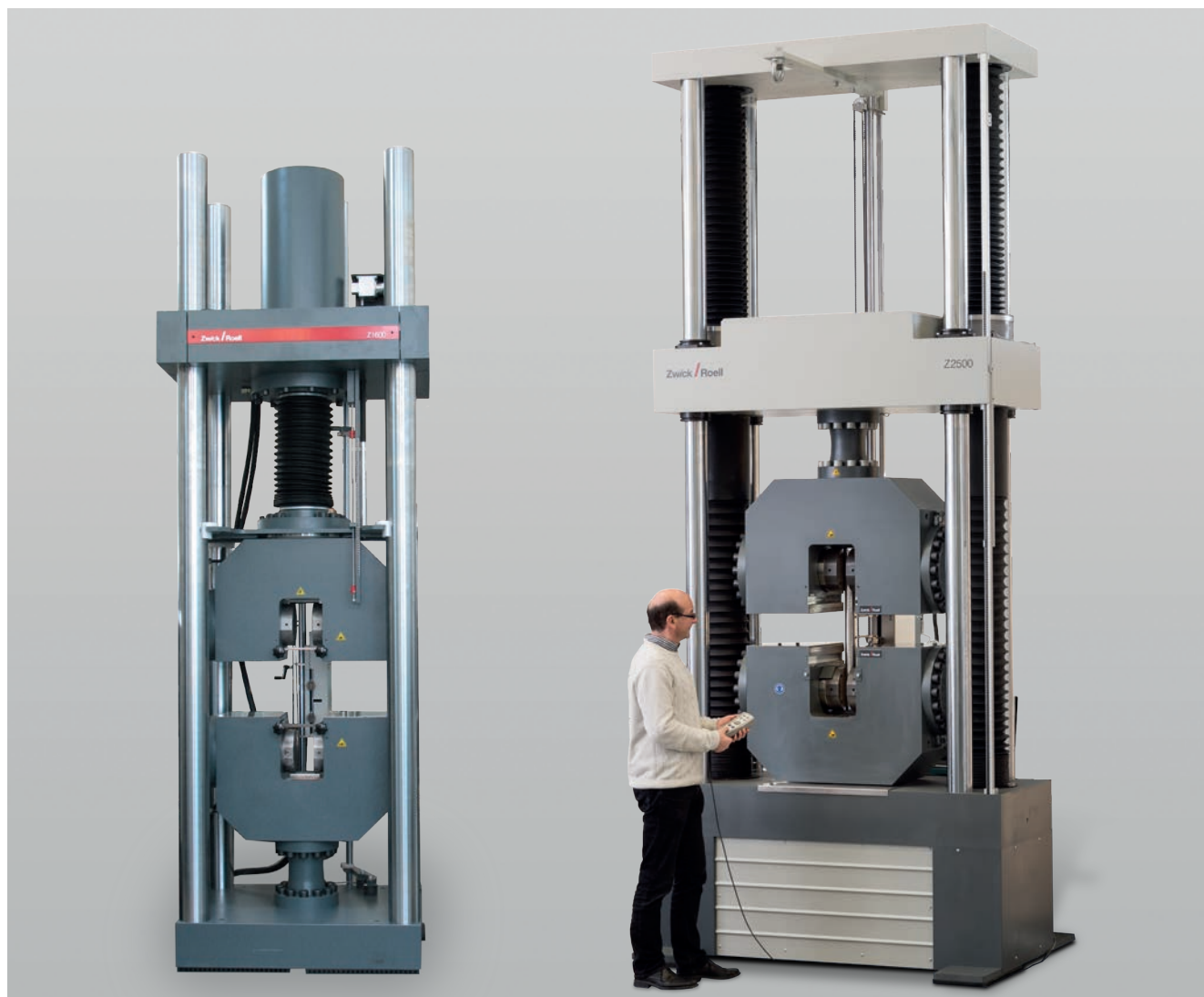
Fig.1: Available from ZwickRoell as standard - high-capacity testing machines up to 2,500 kN
