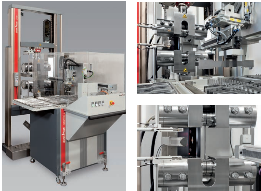
Fig. 1: roboTest L for automated tensile tests on sheet metals
