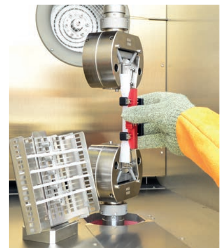
Fig. 3: Optional magazine for preconditioning of specimen.
