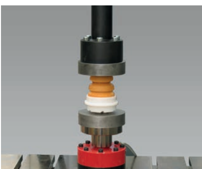
Fig. 4: Dynamic tests on acoustic floor panels and end-cushioning parts
