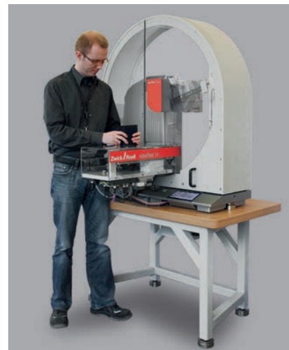
Fig. 3: Specimen feeding for Charpy and Izod - 'roboTest H'
