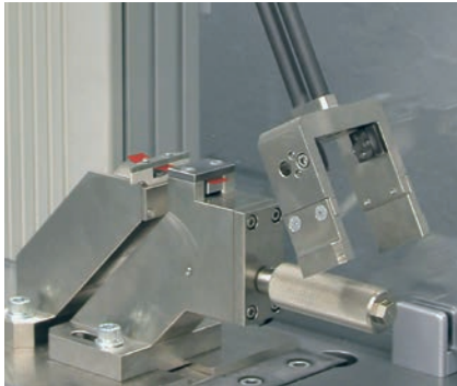
Fig. 3: Tensile-impact test, ISO method A
