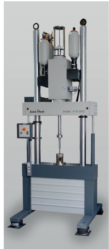
Fig. 3: HTM high-speed testing machine
