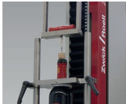
Fig. 6: Extraction tests on bottle corks
