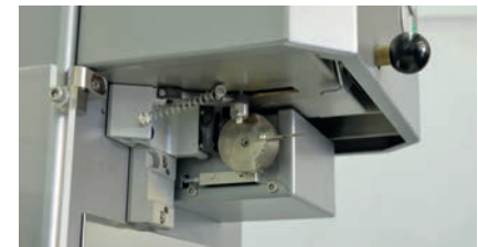
Fig. 3: Extrudate cutter and die-plug
