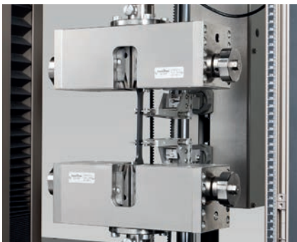
Fig. 3: Mechanical grips with load-dependent clamping for reliable clamping of soft and brittle materials
