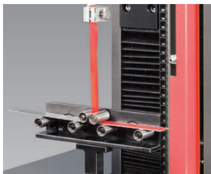
Fig. 1: 90° peeltest to measure peel resistance
