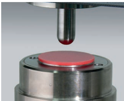
Fig. 4: Multi-axial impact test to ISO 6603-2 with force-travel recording
