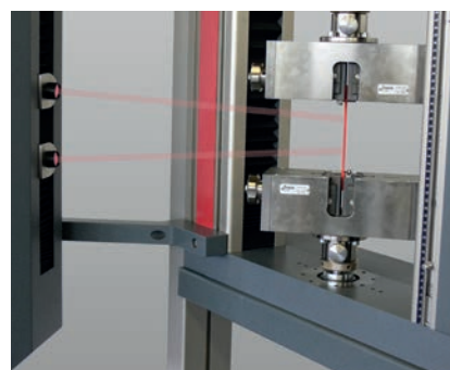
Fig. 6: lightXtens - optical long-travel extensometer
