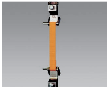
Fig. 4: Grips for specific materials and specimen shapes: ring testing device, toggle grips
