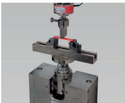
Fig. 4: Easy changeover from tensile to flexure via mechanical slots and setting gages
