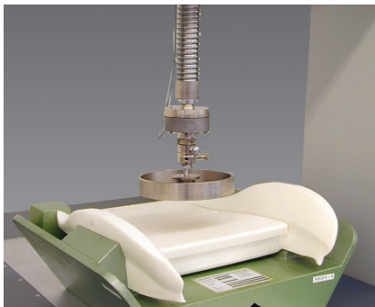
Fig. 3: Indentation hardness of molded foam parts (DIN 53579-1)
