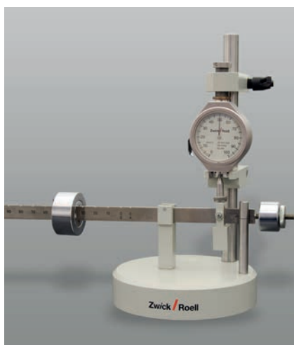
Fig. 1: Shore A and D calibration stand
