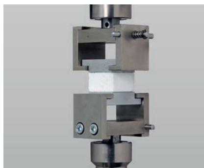
Fig. 4: Perpendicular tensile as per EN 1607
