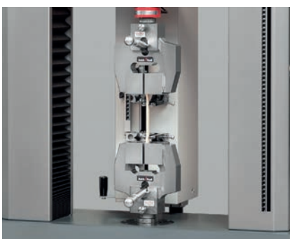
Fig. 4: Mechanical long-travel extensometer
