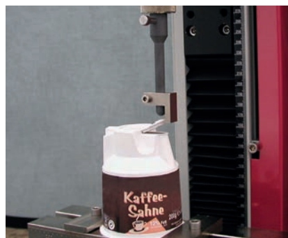
Fig. 5: Determining operating forces
