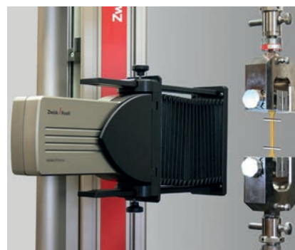
Fig. 5: videoXtens HP for optical measurement of longitudinal and transverse strain
