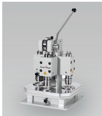
Fig. 2: 7101 eccentric cutting press with centering spigot for circular specimens
