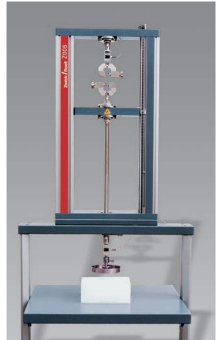
Fig. 2: Testing foam components in the third test area below the load frame
