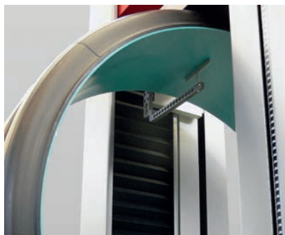
Fig. 1: Measuring ring stiffness, ISO 9969: ring deformation is measured on the internal diameter
