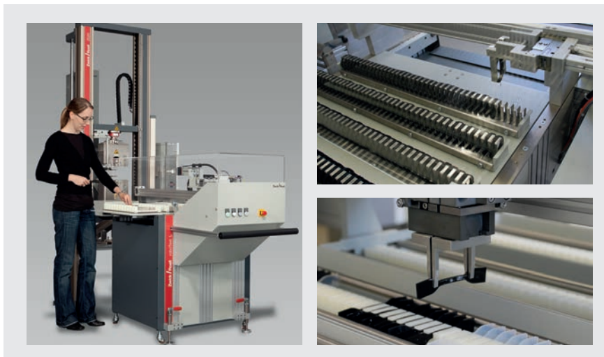
Fig. 1: 'roboTest L' - tensile and flexure tests on plastics and rubber. The large specimen magazine allows operation overnight and at weekends.
