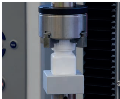
Fig. 7: Function test on safety screw-closures
