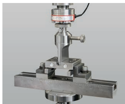
Fig. 4: Easy changeover from tensile to flexure via mechanical slots and setting gages
