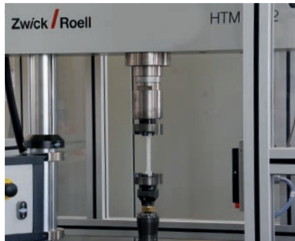
Fig. 3: The high-speed tensile test delivers tensile properties at elevated strain rates
