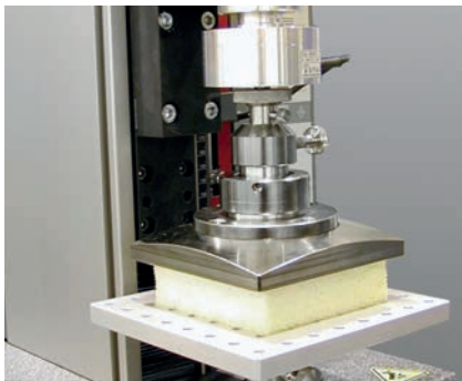
Fig. 1: Compression properties, compression stress value (ISO 3386, ASTM D 3574)
