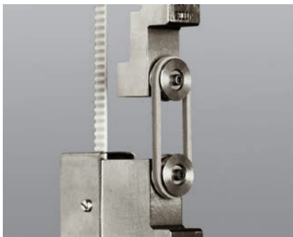
Fig. 4: Grips for specific materials and specimen shapes: ring testing device, toggle grips
