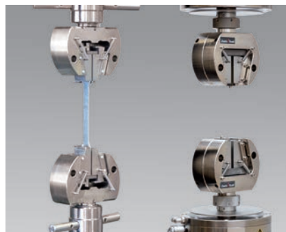
Fig. 6: The Modular BoW gripping system allows easy change of configuration
