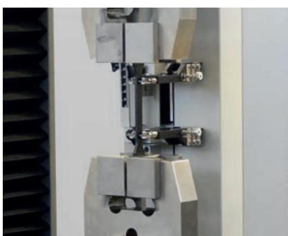
Fig. 4: Tensile test to ISO 6259: specimen shapes depend on wall thickness
