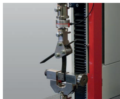
Fig. 5: Floating roller peel test, ISO 4578
