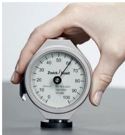
Fig. 2: Analog Shore hardness tester
