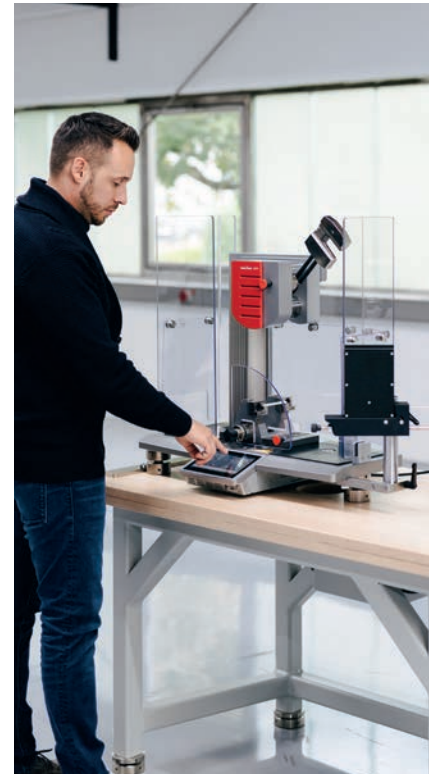
Fig. 2: HIT5P pendulum impact tester
