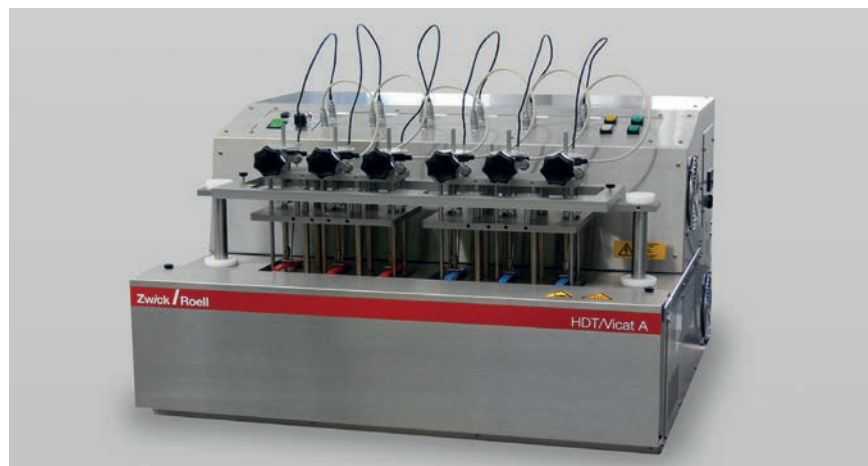
Fig. 2: Allrounders HDT/Vicat 3-300A and 6-300A are fitted with a hoist, enabling the entire test to run automatically. They are equipped with a bath to accommodate three or six measuring stations.
