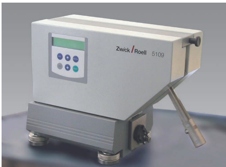
Fig. 1: ZwickRoell 5109 rebound resilience tester with digital display
