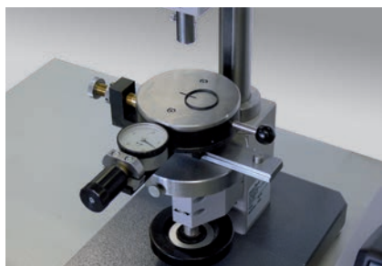
Fig. 2: Hardness test on O-rings
