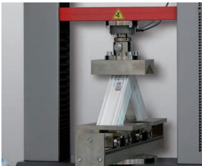
Fig. 3: Corner strength of a window frame
