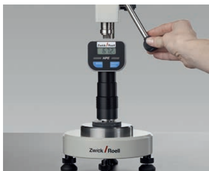
Fig. 2: Shore A hardness, ISO 48-4
