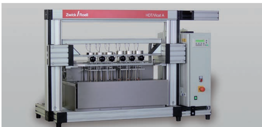
Fig. 1: The HDT/Vicat 3-300 A and 6-300A with integrated heat exchanger and three or six measuring stations.
