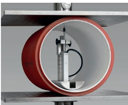
Fig. 2: Special displacement transducers are available for pipes up to 630 mm diameter
