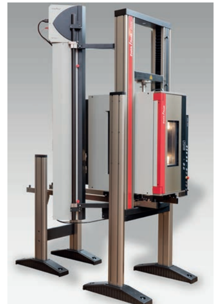
Fig. 2: The temperature chamber can be slid out on rails
