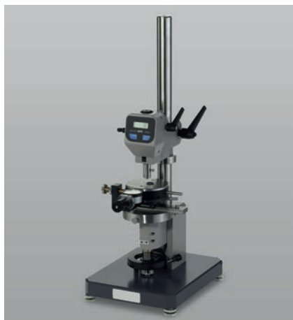
Fig. 1: ZwickRoell 3103 IRHD micro compact
