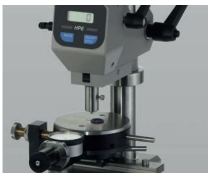
Fig. 6: IRHD hardness of an O-ring
