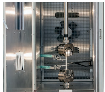
Fig. 4. Temperature chambers can also be retrofitted
