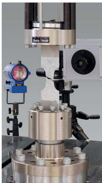
Fig. 2: High-speed tensile test with a test speed of up to 20 m/s
