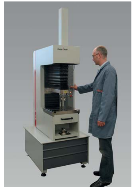
Fig. 5: Push out test for riveted joints
