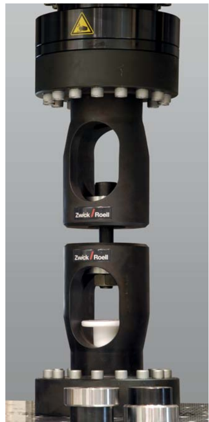
Fig. 2: Fatigue tests on threaded connections with the Vibrophore
