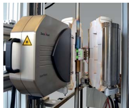
Fig. 4: High-temperature furnaces can also be retrofitted
