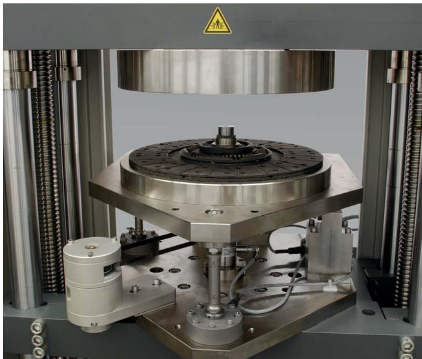
Fig. 1: Determination of contact force and displacement as well as push out force and displacement of friction clutches
