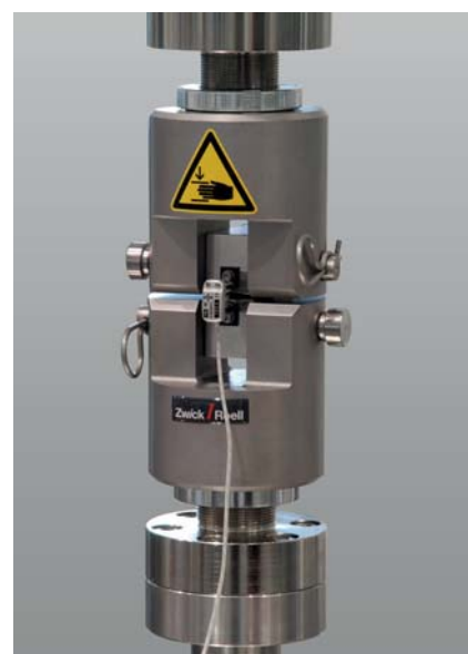
Fig. 2: Determination of the fracture toughness K_{Ic}
