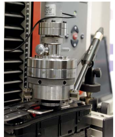
Fig. 3: Acoustic-haptic tests on multi-function rotary switches
