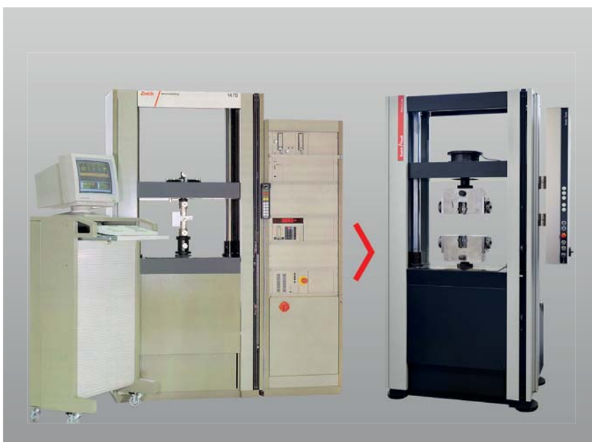
Fig. 1: Modernization of a static testing machine with testControl II
