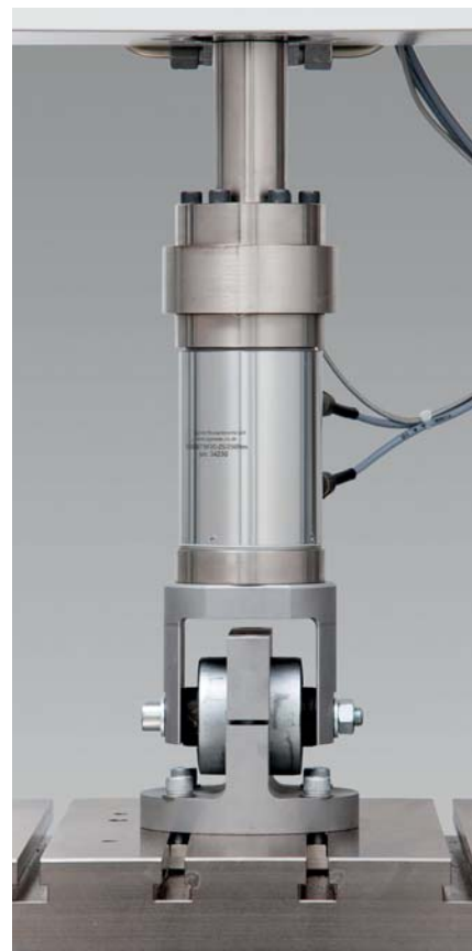
Fig. 3: Testing of rubber-metal dampers
