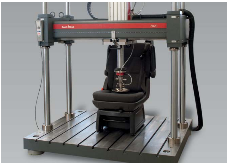
Fig. 2: Flexible test bench for characterizing seats
