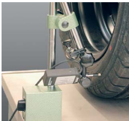
Fig. 2: Axial, horizontal forces and tire pressure are controlled via testControl
