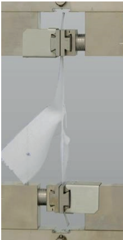
Fig. 1. Tear growth test on textiles
