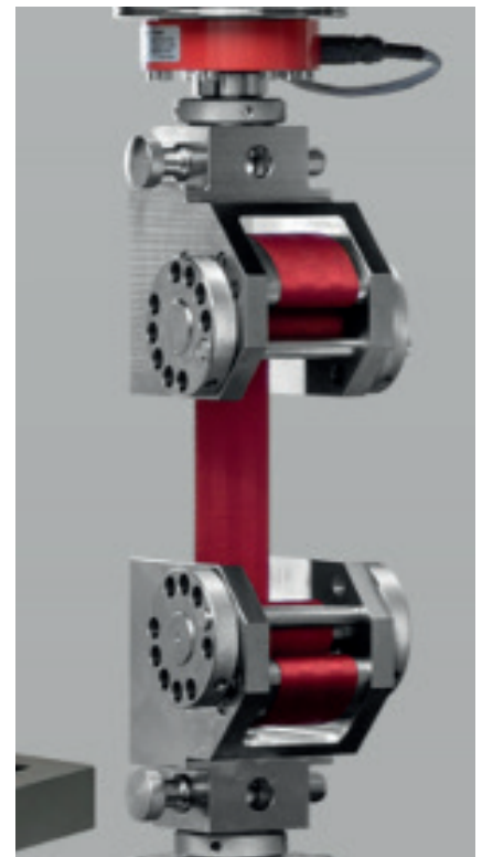
Fig. 2. Tensile test on belts
