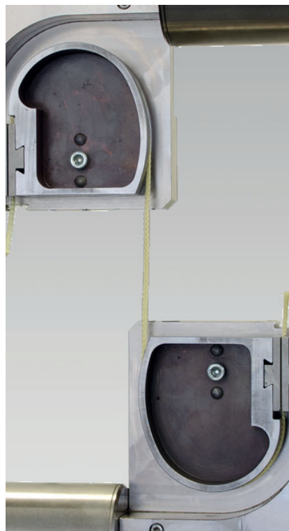
Fig.2. Tensile test on two-ply yarn
