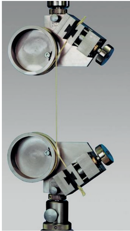
Fig.1. Tensile test on multi-filament yarn
