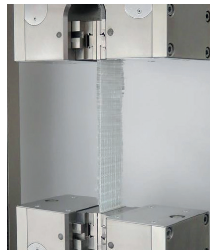
Fig. 3. Tensile test on woven textile glass fabric
