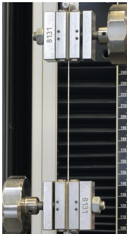
Fig. 1. Tensile test on sewing yarn
