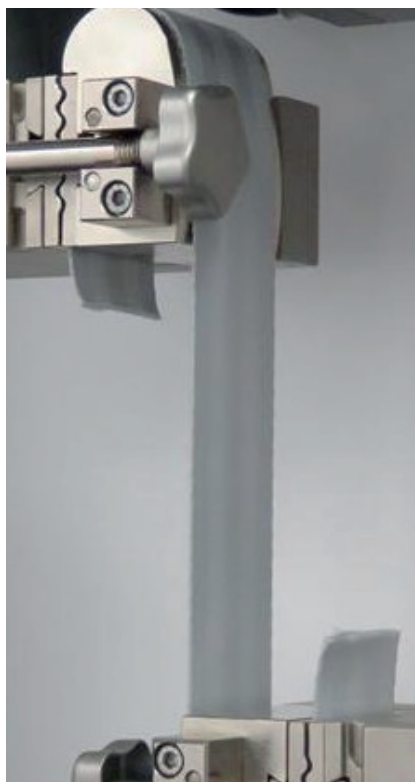
Fig. 1. Tensile test on textile fabrics
