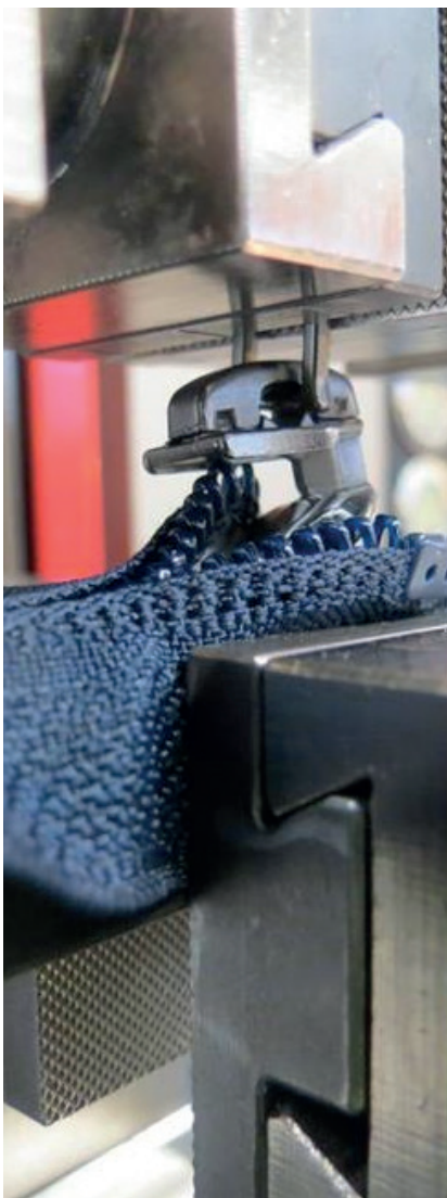
Fig. 1. Tensile test on zip fasteners
