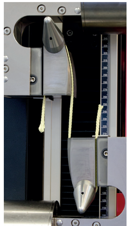
Fig. 2. Tensile test on aramid yarn
