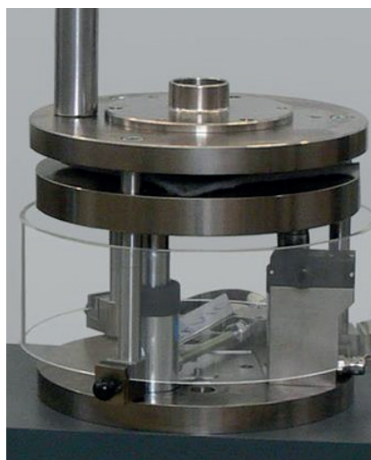
Fig. 2. Static puncture test (CBR test)
