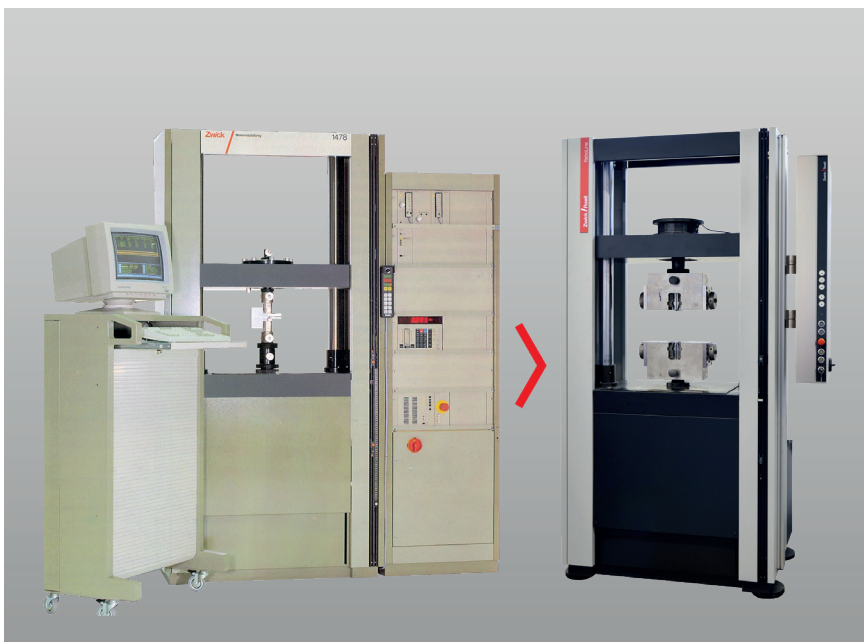
Fig. 1. Modernization of a static materials testing machine with testControl II
