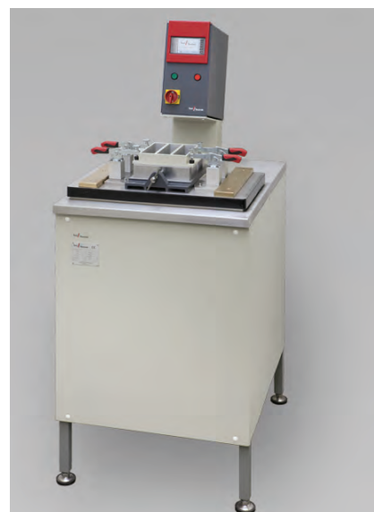
Fig. 3: Vibrating table for standard-compliant specimen compacting (controlled)
