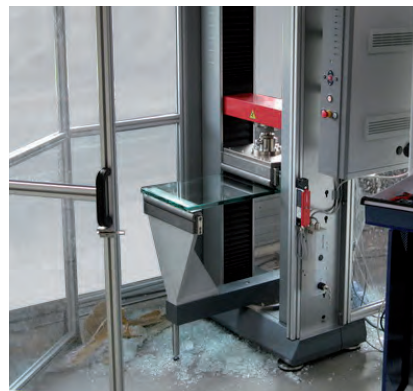
Fig. 3: 4-point flexure test on construction glass
