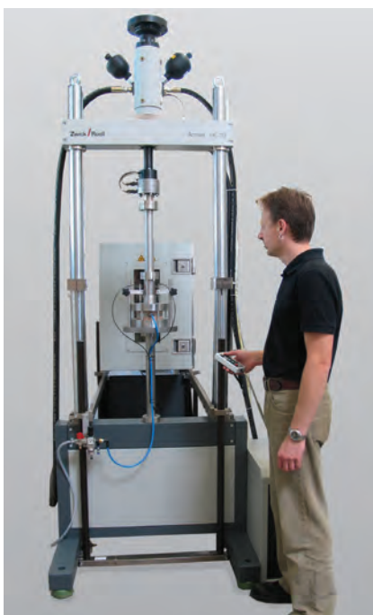
Fig. 1: Servo-hydraulic testing machine with temperature chamber
