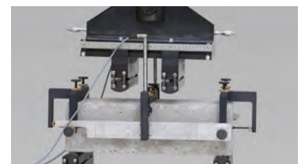
Fig. 4: Deformation transducer for measuring deflection
