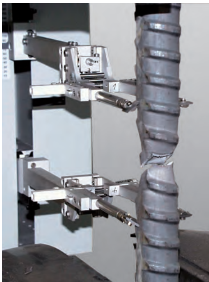
Fig. 1: Tensile test on ribbed reinforcement steel using Makro extensometer
