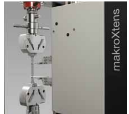
Fig. 3: Mechanical measurement, automatic attachment: makroXtens
