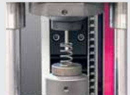
Compression test of springs
