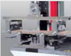
4-point flexure test of cardboard
