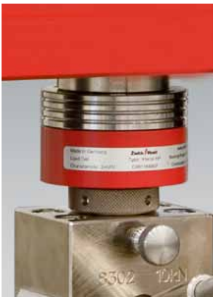
Fig. 1: Load cell from the Xforce range employing multiple beams
