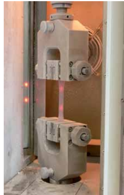
Fig. 3: Tensile test at 70 °C with optical strain-measurement
