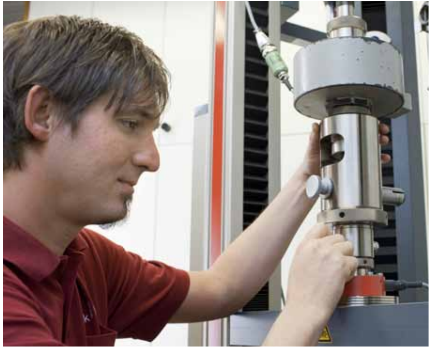
Fig. 2. Every load cell is calibrated by Zwick as soon as it is put into service on a testing machine
