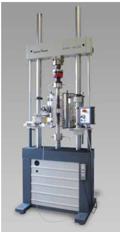
Fig. 1: Fatigue test at high temperature
