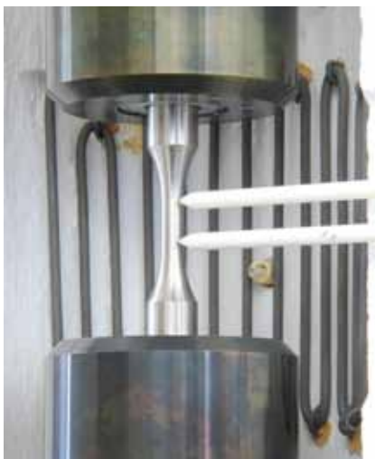
Fig. 1: LCF test at high temperature with extensometer attached
