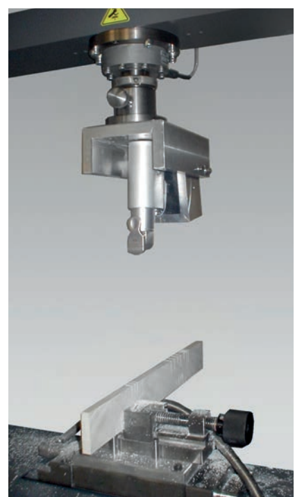
Fig. 3. Compression test on sagittal saw blade
