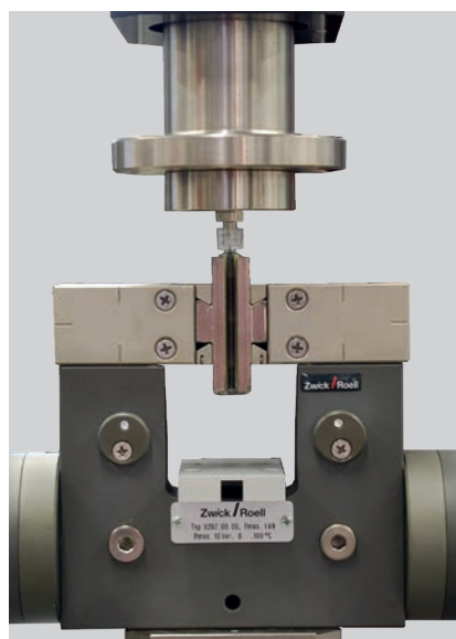
Fig. 3. Testing luer lock connections
