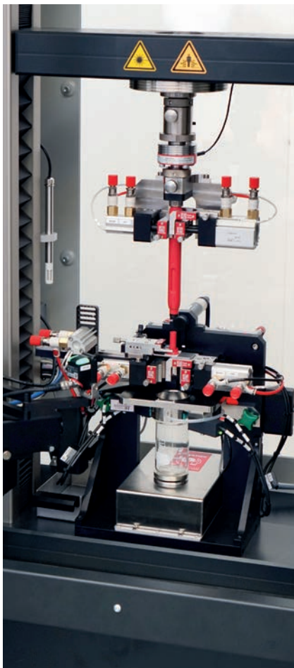
Fig. 1. Multiple tests on autoinjectors
