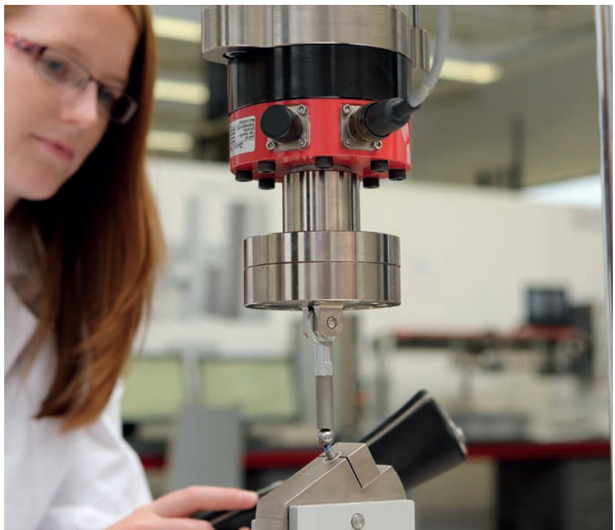
Fig. 1. Fatigue test on dental implants
