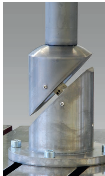
Fig. 2. Torsion test on vertebral body implant
