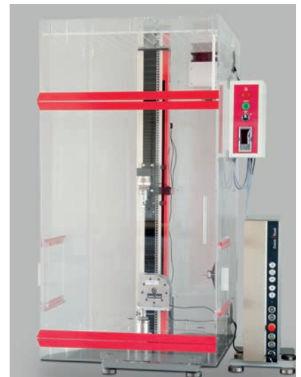
Fig. 3. Temperature chamber installed with a materials testing machine
