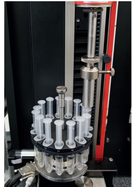
Fig. 3. Semi-automatic test on syringes
