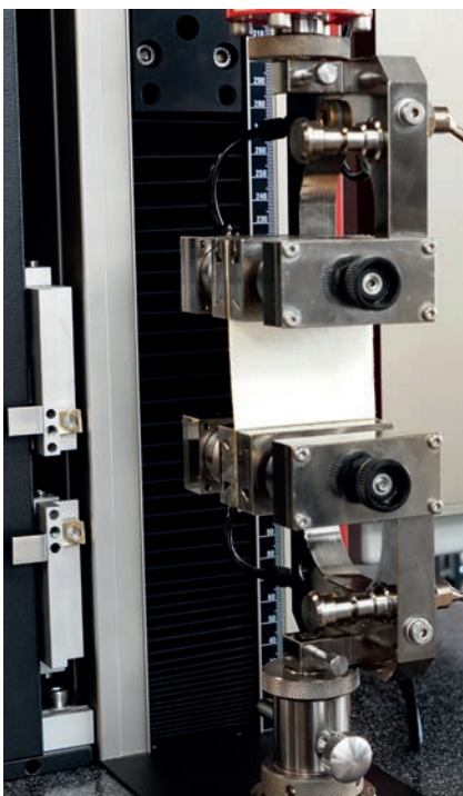
Fig. 1. Tensile test on medical textiles
