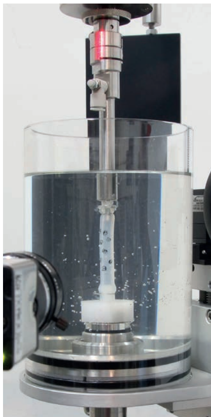
Fig. 1. Triaxial test on tissue using torsion
