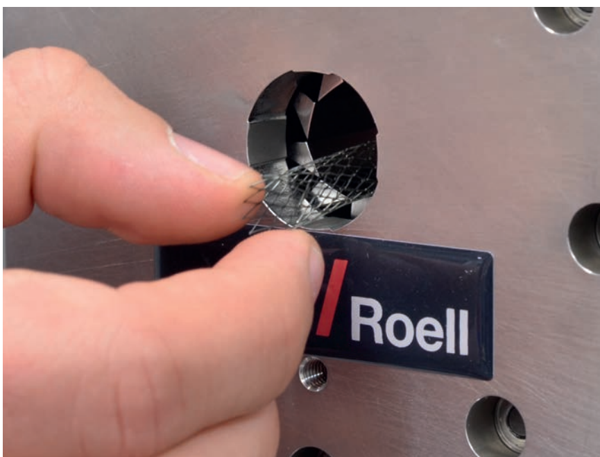
Fig. 1. Radial compression tests on stents
