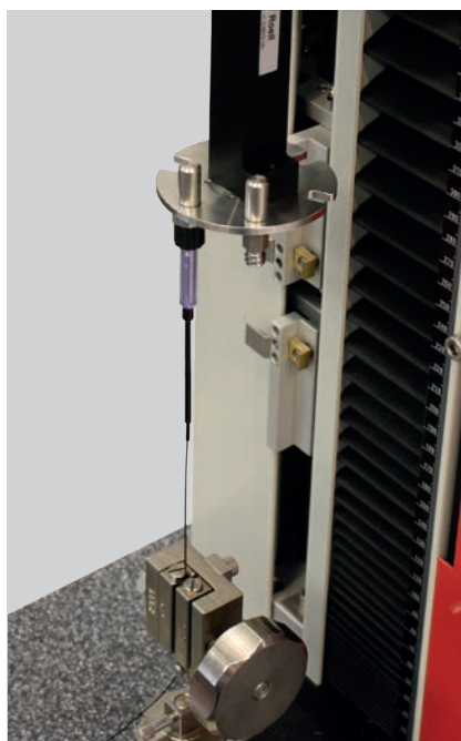
Fig. 2. Tensile test on catheter systems
