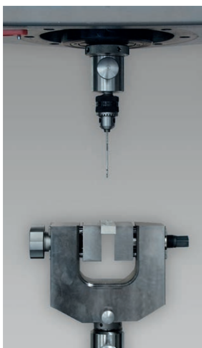
Fig. 2. Penetration test for a bone drill
