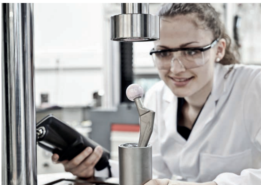
Fig. 1. Fatigue test on hip prosthesis
