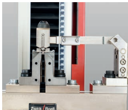
Fig. 3: Standard 10 mm adjustment gauge for exact alignment
