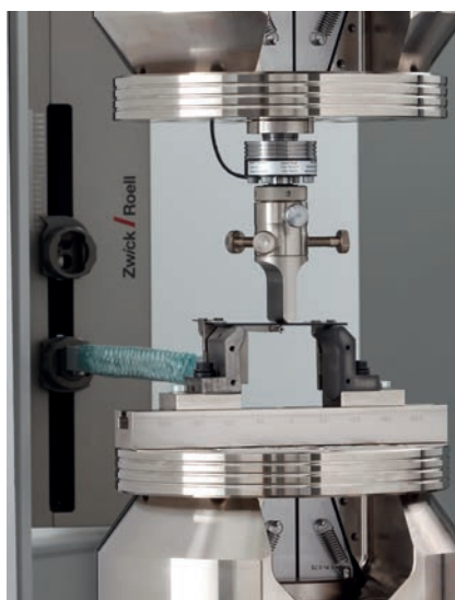
Fig. 3: makroXtens with flexure sensors for 3- and 4-point flexure tests
