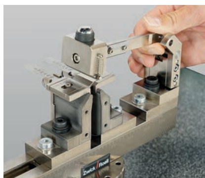
Fig. 4: Adjustment gauge with variable support span
