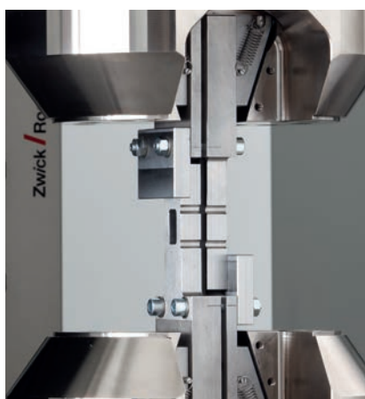
Fig. 5: OHC and FHC compression tests to ASTM require an anti-buckling support, which is used for shear loading with hydraulic specimen grips, and with end loading between compression platens.
