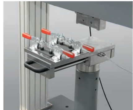
Fig. 3: Secure mounting of the CAI specimen in the drop weight tester
