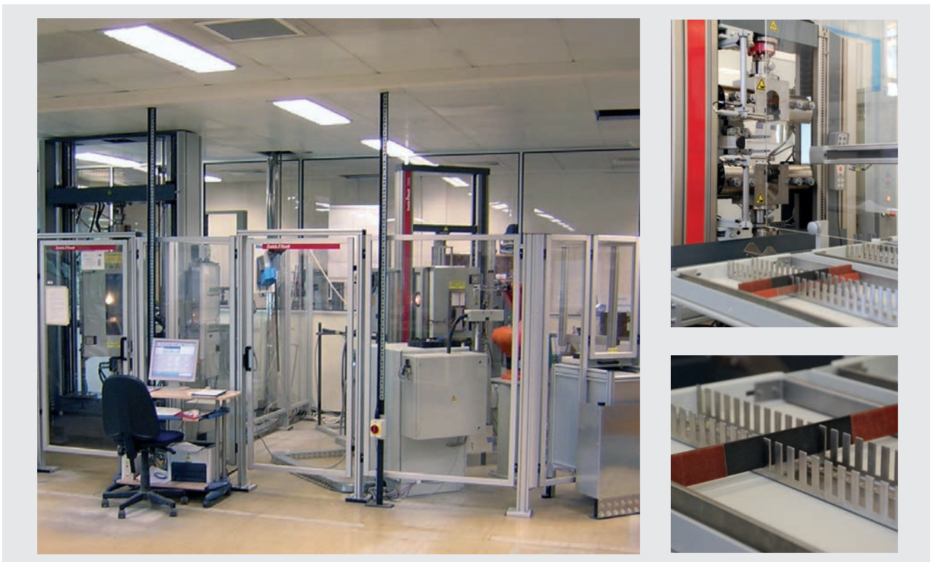
Fig. 1: Fully automated testing system with two load frames for tensile, OHT, FHT, IPS, lap shear, ILSS, bearing response and flexure tests over a wide temperature range
