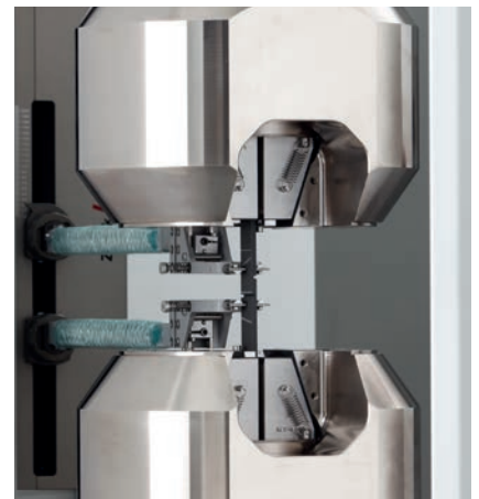
Fig. 1: For testing of laminates, centrally closing wedge grips, side adjustable wedge screw grips, as well as hydraulic, parallel closing body-over-wedge grips with a wide selection of jaws, are available.
