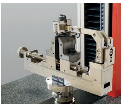
Fig. 1: Support and die are exactly parallel. Centering stops make operation easy.
