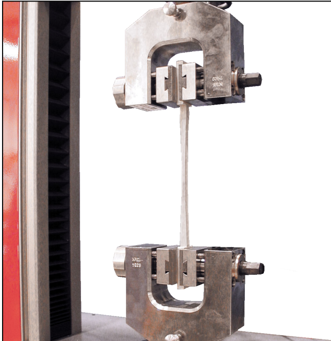
Screw grips, Type 8354, Fmax 10 kN
