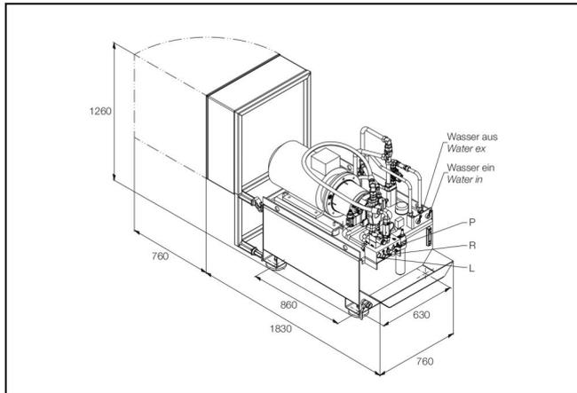
Hydraulikaggregat 20 Liter
