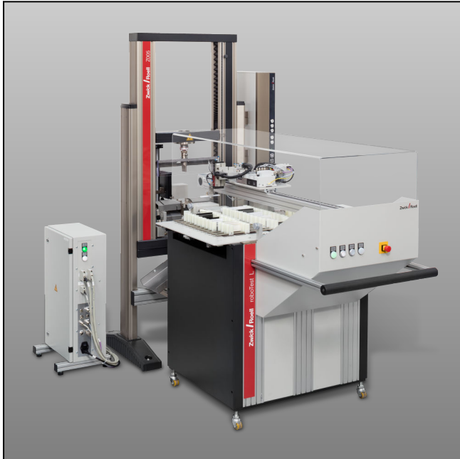
roboTest L robotic testing system for plastics
