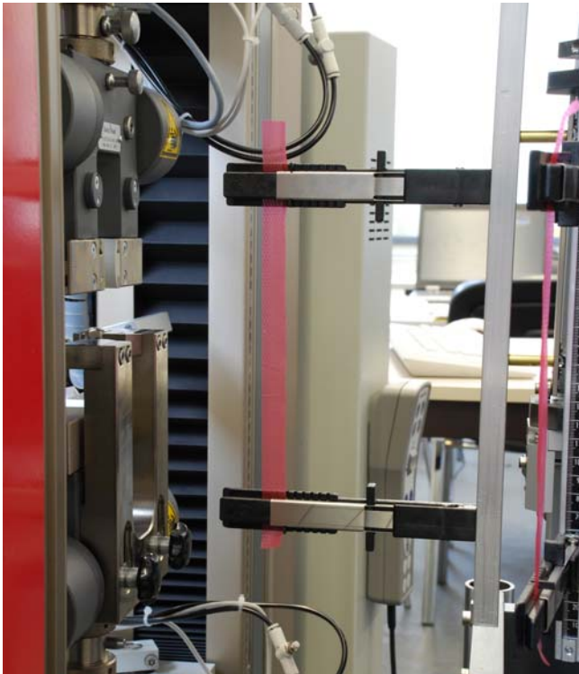
Feeding of a strip specimen to the materials testing machine
