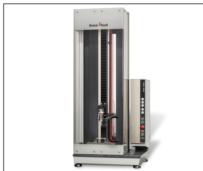
Swivelable front safety device, with electrical interlocking
