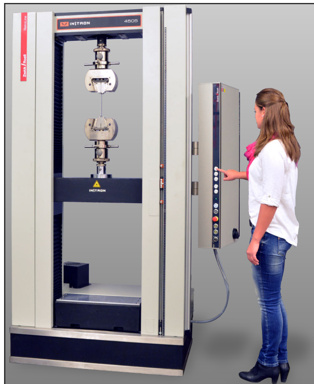
Instron 4505 (100 kN) with new testControl II electronics
