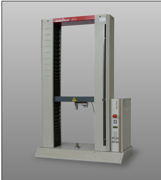
ProLine Z10 with MOPS electronics before modernization
