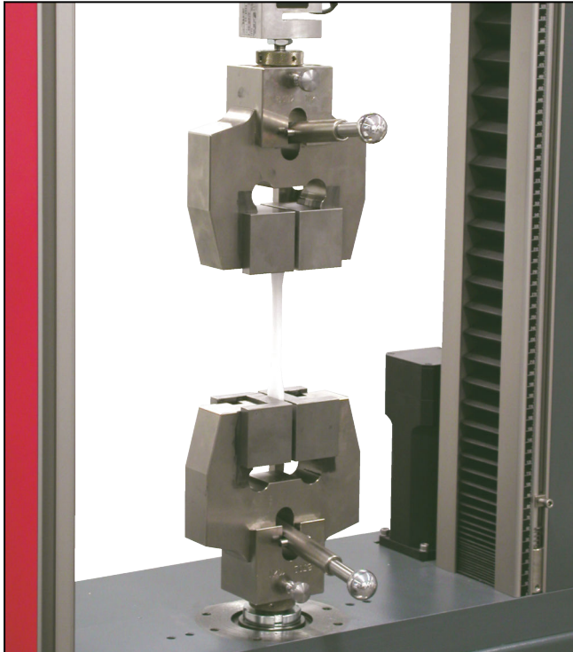
Wedge grips type 8302, Fmax 10 kN
