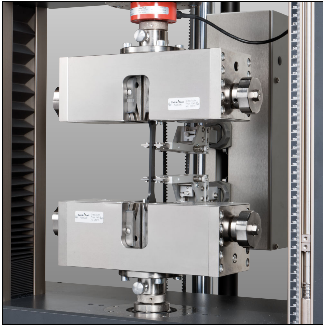
Type 8306 wedge screw grips, Fmax 10 kN
