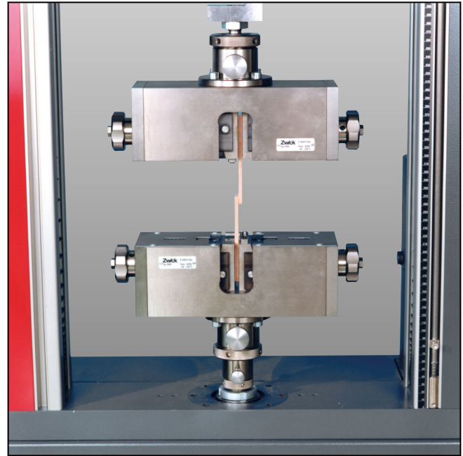
Type 8406 wedge screw grips, Fmax 30 kN
