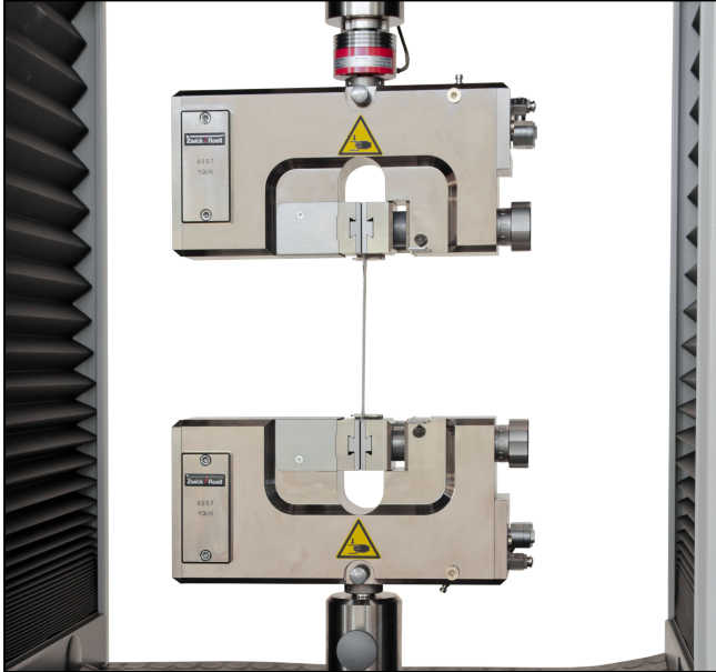
Pneumatic grips type 8397, Fmax 10 kN
