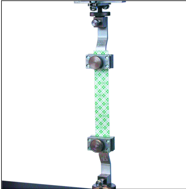
Type 8153 screw grips, Fmax 20 N
