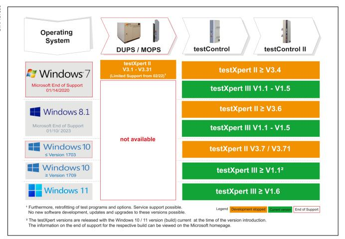
Switching from testXpert or testXpert II to testXpert III
