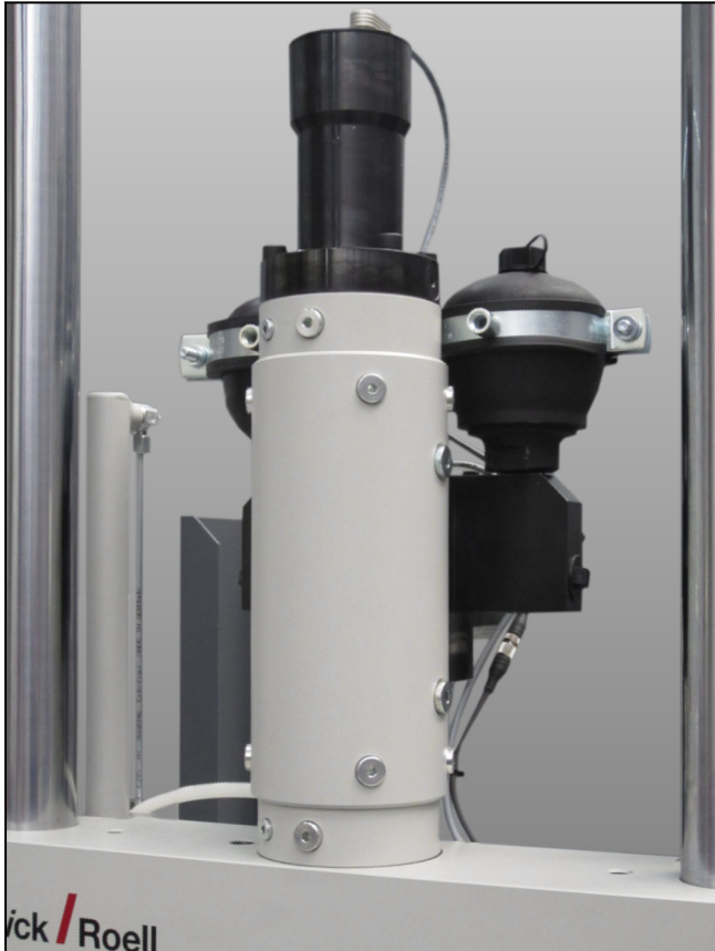
LH actuator, overhead installation in a test frame
