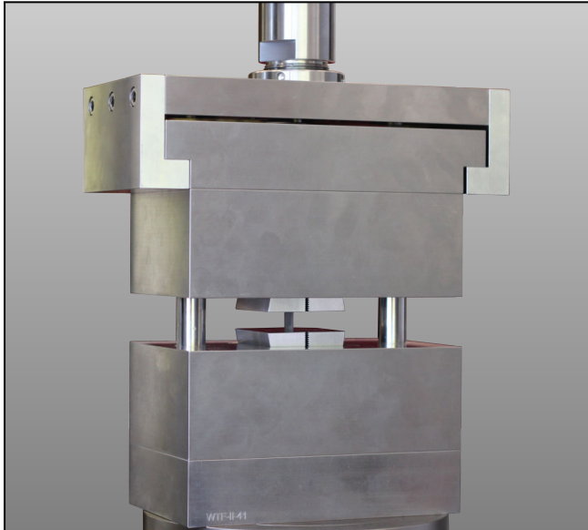
Compression test kit (shear loading), IITRI version
