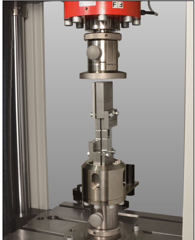
Open-hole compression fixture installed in locking shoe mount; force application via compression platen
