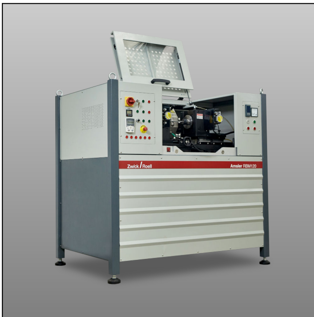
Testing area open – clamping specimen
