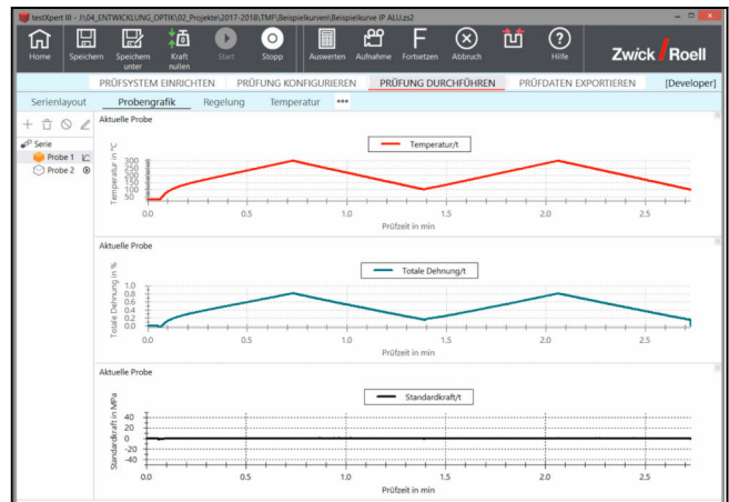
Step 1: Temperature control, stabilization Step 2: Determination of thermal strain
