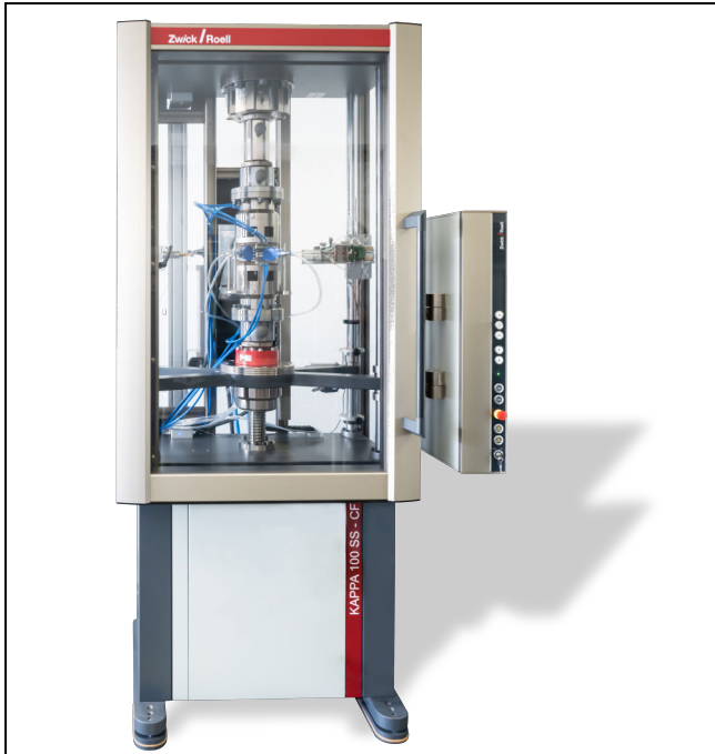
Thermomechanical fatigue testing system
