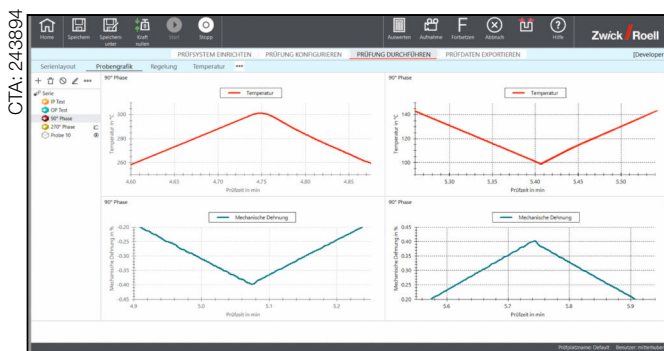
Upper and lower temperature reversal point (red), upper and lower reversal point of the mechanical strain (blue)
