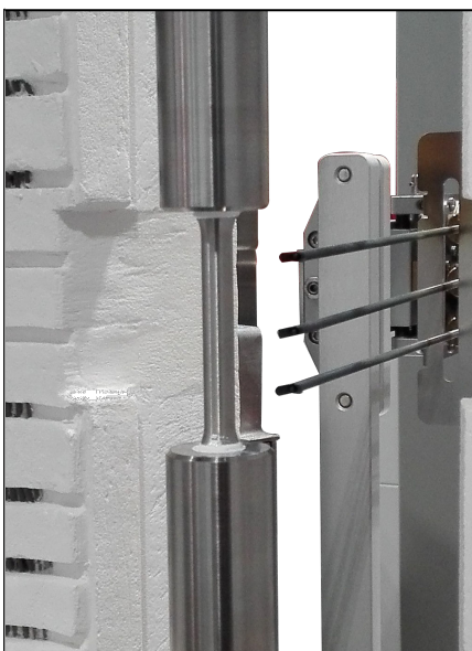
I) High-temperature specimen adapter for round specimens with threaded head and variable thermocouples (not attached)
