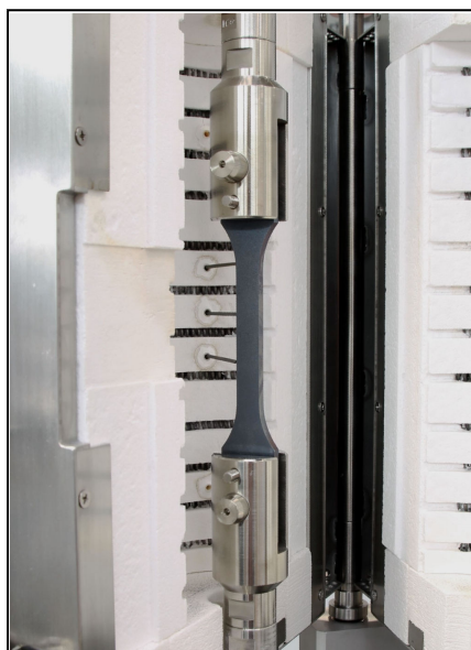
II) High-temperature specimen adapter for shoulder-end specimens with hole and fixed thermocouples (attached)
