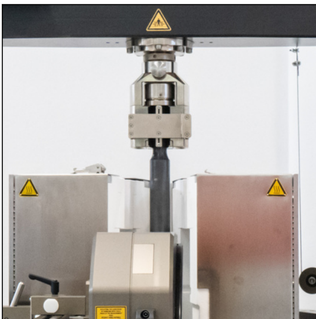
High-temperature pull rod coupling for universal testing machines
