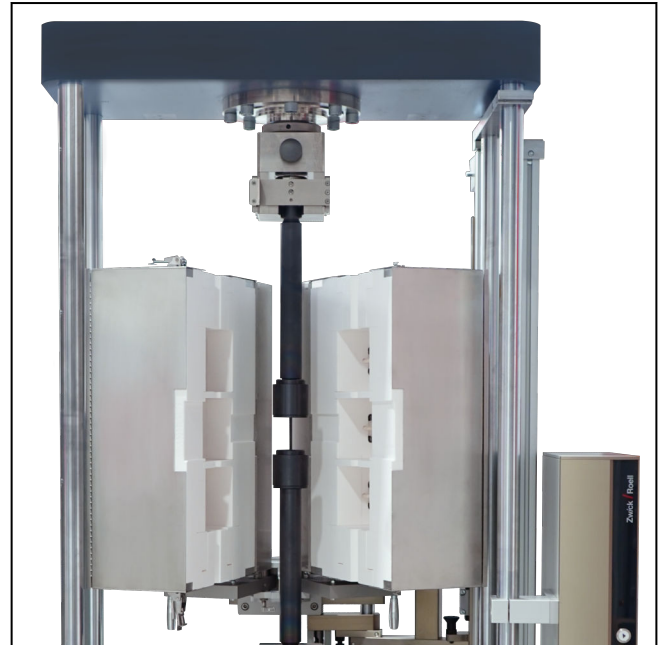
Ceramic load string in creep testing machine Kappa SS
