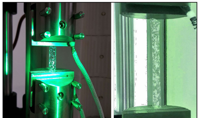
Marked glass specimen before (left) and after (right) the high-temperature tensile test
